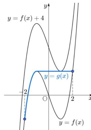
$$\begin{aligned} \int_{-2}^2 g(x)dx &= \int_{-2}^{-1} f(x)dx + \int_{-1}^2 2dx \\ &= \left[ \frac{x^4}{4} - \frac{3}{2}x^2 \right]_{-2}^{-1} + [2t]_{-1}^2 \\ &= \left( -\frac{5}{4} + 2 \right) + 6 \\ &= \frac{27}{4} \end{aligned}$$
